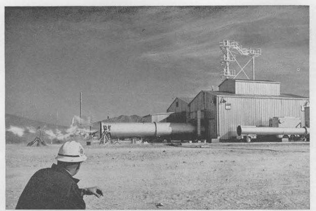
SHOCK TUBE belches a sheet of flame at moment of detonation of high-explosive charge during acceleration test in Area Y. Bob Allison (7423-2) observes the
